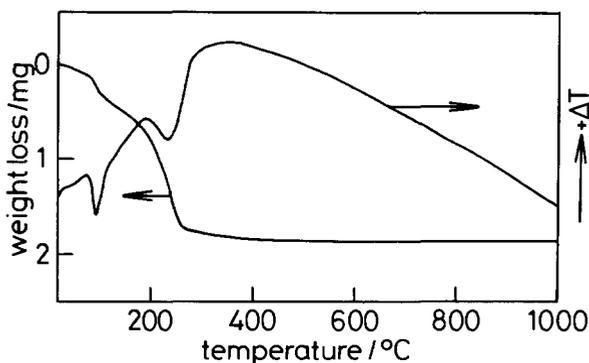
Fig. 2. Results of thermal analysis for the zinc oxide carbonated at 8°C for 14 days. Starting weight: 5.071 mg.
