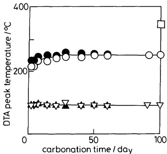
Fig. 4. Dependence of DTA peak temperature on the carbonation period. ▽, ○ and □, carbonated at 8°C; ▲ and ●, carbonated at 13°C; ▽ and ▲, the first endothermic peak at ~90°C; ○ and ●, the second endothermic peak at ~220–250°C, □, the third endothermic peak at ~340°C.
