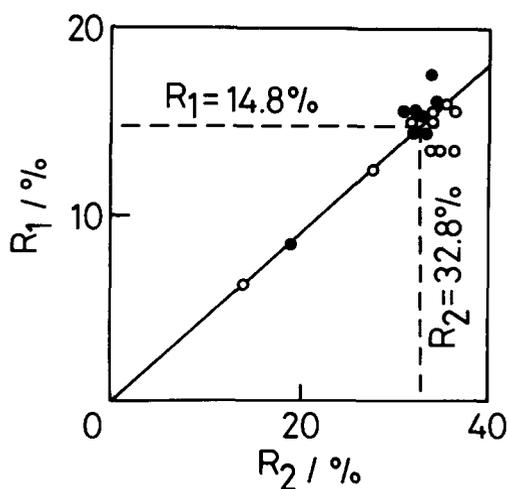
Fig. 6. Relation between  $R_1$  and  $R_2$ :  $\circ$ , carbonated at  $8^\circ\text{C}$ ; and  $\bullet$ , carbonated at  $13^\circ\text{C}$ .  $R_1$  and  $R_2$  are defined in the figure caption of Fig. 5.
