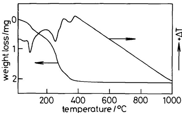
Fig. 3. Results of thermal analysis for the zinc oxide carbonated at 8°C for 100 days. Starting weight: 5.245 mg.
